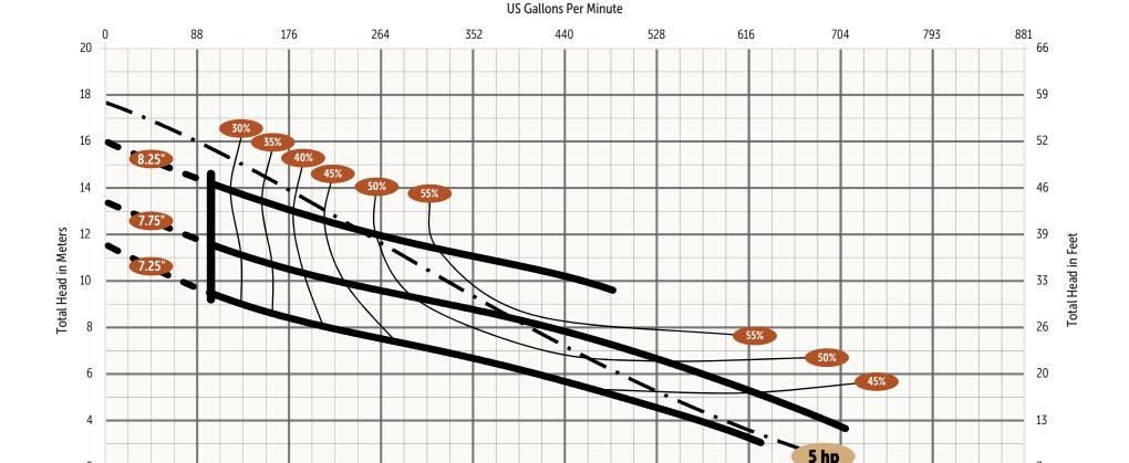
Stated efficiency values are hydraulic efficiency. Wire-to-Water (total) efficiency information is available upon request.
